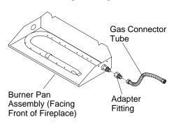
Figure 10 - Connecting Gas to Appliance
